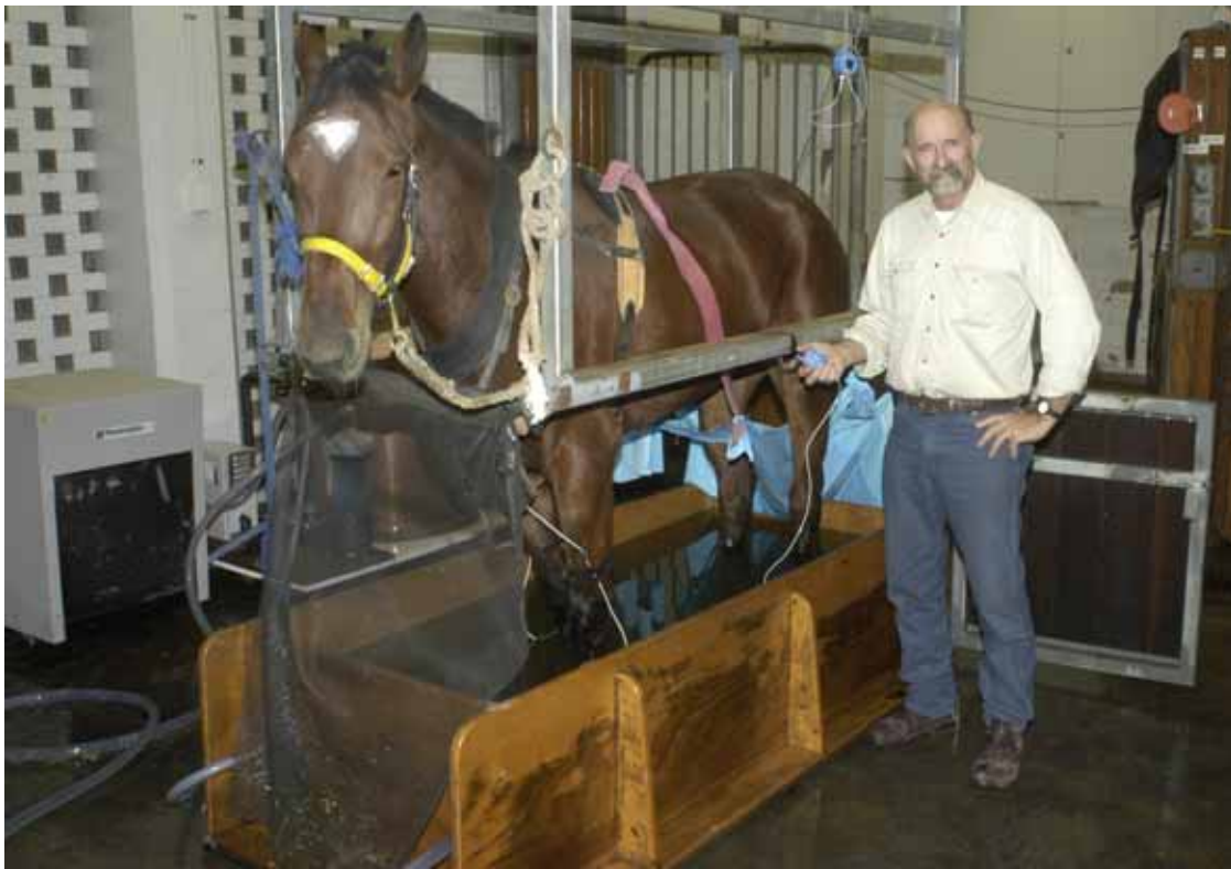
Figure 2. Experimental set-up showing a horse is restrained standing in a tub of marine ply construction for prolonged, continuous application of cryotherapy to all four limbs. There is a water-tight door at one end for ease of access and a rubber floor. The horse is cross-tied standing in cold water to the proximal cannon level. A refrigeration unit and pump, against the far wall, are cooling and re-circulating water at around 2°C. Plastic sheeting prevents food, faeces and urine from contaminating the water and blocking the pump filters.
